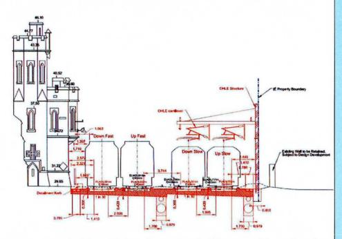
seems open to interpretation. For example this excerpt from Drawing DP-04-23-DWG-RO-TTA-18984 states existing wall to be retained 'subject to detail development.' Furthermore this section does not convey the foundational work associated with the OHLE mast which is shown to sit directly on the IE property boundary.
